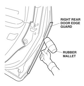
12. Repeat step 8 through 11 to install the le door edge guard.
